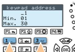
During the addressing phase, do not exceed the maximum number of addresses available for the control panel model you are installing. For the readers addressing, use keypad "1".
