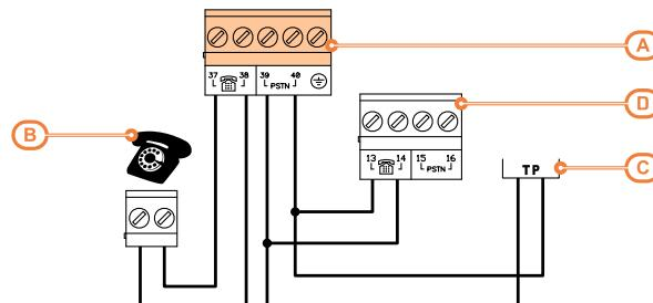
If you are installing the control panel in a place where the land line (PSTN) service is not available, or if you wish to increase the level of security of the system, these terminals also accept a GSM interface (such as SmartLinkAdv) which simulates the analogue land-line.
