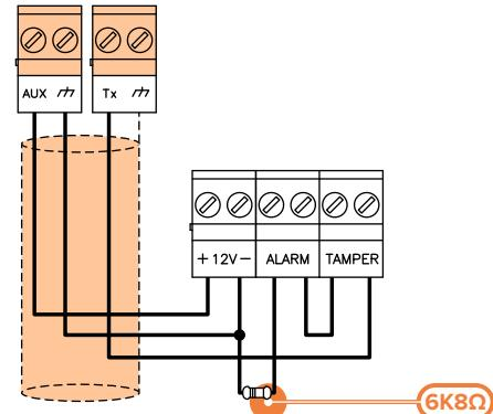
If you wish the detector to signal tamper events, it is advisable to connect the "Tamper" terminal to a "24h" zone on the control panel.
