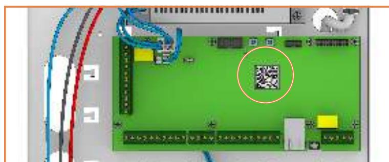
2. The Prime control panel has a unique QR-code relating to the serial number of the control panel in use.
