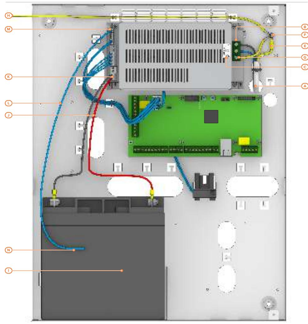
1. Pull the power-supply cables through the cable entry [A].
