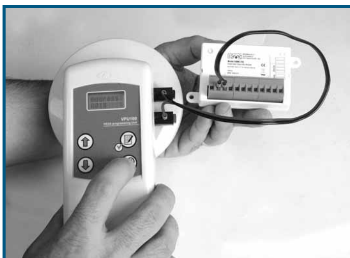
Figure 34 - Addressing modules using a VPU100
